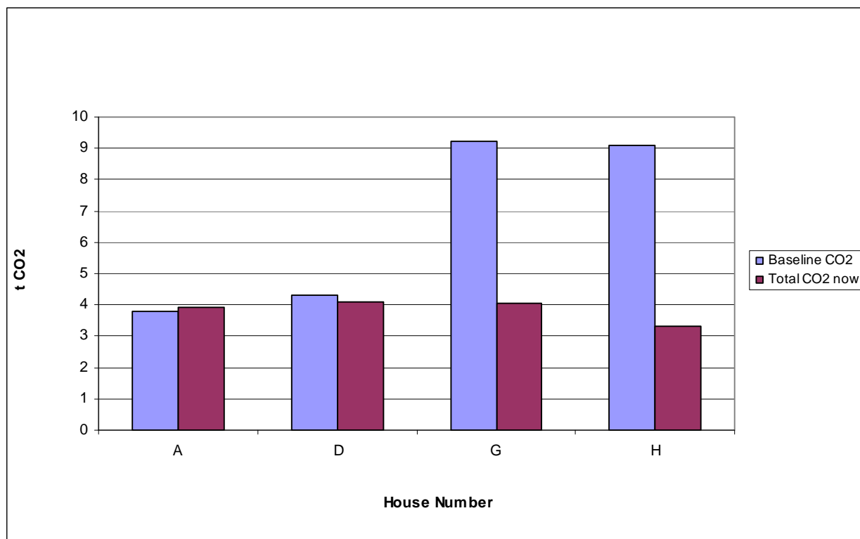
Figure 4.1 Carbon emissions pre- and post-GSHP installation
